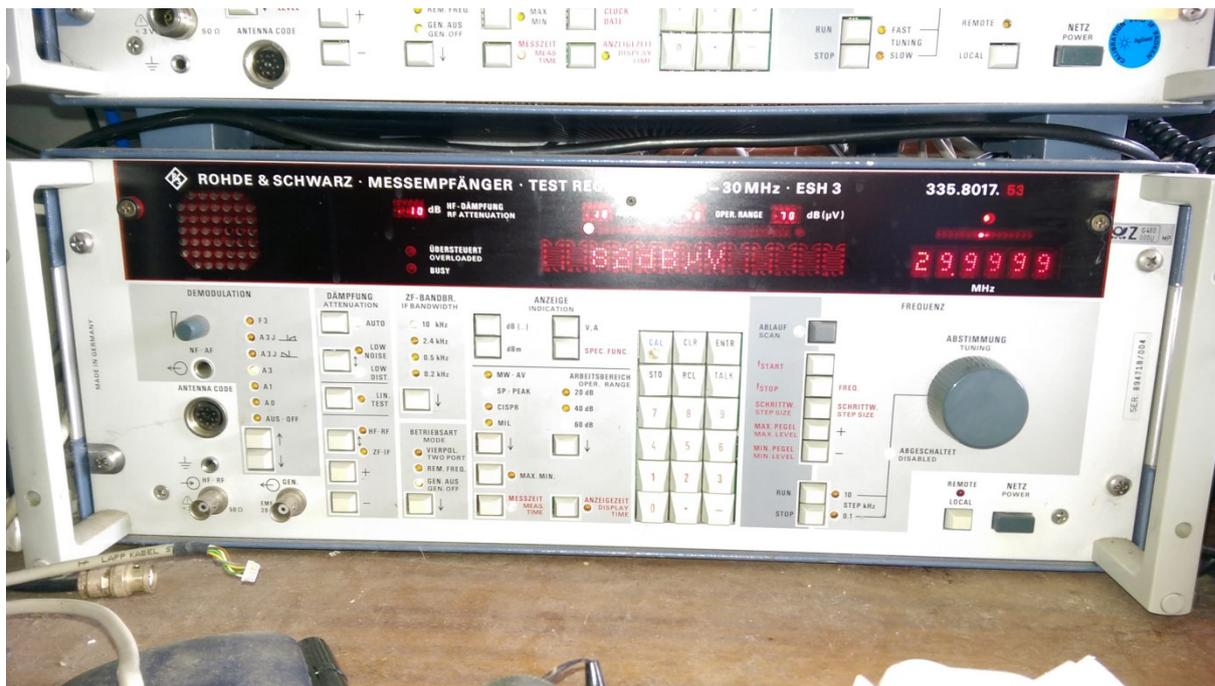
9kHz to 30MHz Test Receiver.
