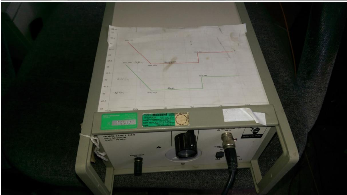
This is used to safely and accurately measure the amount of interference injected into the mains supply by the device under test.
